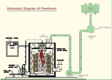
Most of our manufacturing units use Thermic Fluid Heater for process heating. Accidents due to improper handling/maintenance of Thermic Fluid Heater are not uncommon and the following precautionary measures should be taken to prevent any untoward incident:
