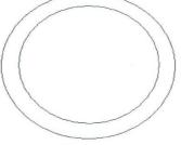
MATERIAL; P.B. WITH OIL GROOVE INSIDE AREA OD, ID GRINDING FINISHING REQUIRED ALL DIMENSIONS ARE MM
